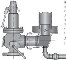
**Model 299** Illustration shows a discharge elbow and drip pan unit attached to a safety valve with female NPT outlet. For safety valves with flanged outlets – 2" to 4" – use companion flange, short nipple and drip pan elbow, all same size as valve outlet. 6" and 8" elbows have integral 125# ANSI B16.1 Flange.
